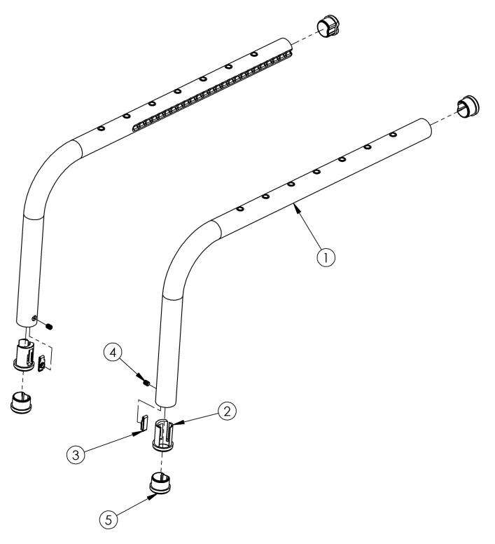
This design effective starting with serial numbers CLK005270. Drilled Clik Side Frames effective April 13, 2018. Replacement side frames may be quoted, but must be ordered through Customer Service. Serial number required upon order.Item numbers 2-4 are only needed when footrest is not high mounted and these parts are included with replacement side frames if footrest is not high mounted.
