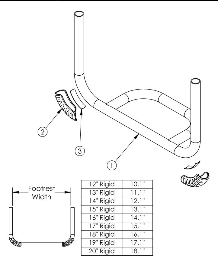
Sizes based on straight frame If changing from a high mount footrest to a frame inserted footrest on a Rogue or Tsunami, please see the appropriate Rigid Frame page for necessary attaching hardware. On Tsunami, if footrest is installed prior to December 2012, new attaching hardware is required.
