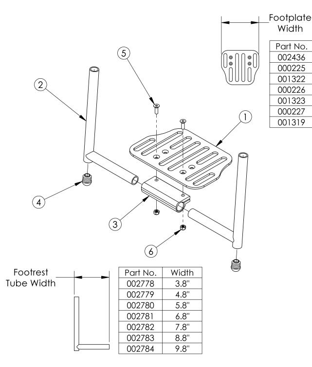
For attaching footrest hardware, reference the Clik Side Frame pages (serial numbers CLK005270 and after) or Discontinued Side Frame pages (serial numbers prior to CLK005270).
