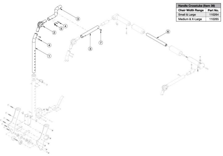
Callout #3: 10"-13" widths receive the curved tube and 14"-18" widths receive the straight shaped tube. When changing backrest types, check to see if new cables and tilt triggers are needed for both foot and hand tilts. If chair was invoiced prior to 12/18/23, an upper back tube assembly is required. If chair was invoiced after to 12/18/23, upper back tube assembly parts can now be purchased individually
