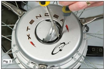
2) Use a 2mm Hex key to loosen the set screw securing the Plate Assembly to the axle.
