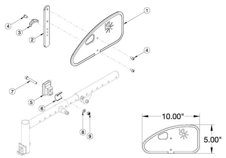
Callout #6: Spacer is needed the when receiver sits on the seat growth tube. Callout #7: Depending upon the placement of the receiver will depend on the length of screw you'll need. More specific information is on the way! Please note there is a receiver screw and spacer kit that includes all potential screw sizes and spacer (you will need qty 2 for a pair).
