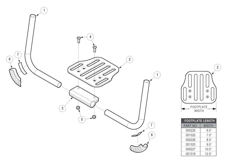
Use Short Footrest if 0" taper and footrest length is 9" - 10.5" or if 1" or 2" taper and footrest length is 9" - 15.5" See Ethos Seat Frame page for hardware to attach footrest tubes to chair.
