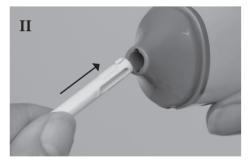
Battery Installation: Remove plastic from included battery. To open battery compartment (located on bottom of device) twist battery cap to the left and pull away from unit. (I) To Insert battery, slide the + terminal inside the unit so it snaps into place. Position cap slightly to the left, push and rotate cap into place. Twist to the right to lock.
