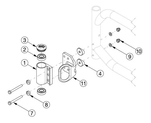
Reference order form for detailed front seat height matrix. Please Note: The shown orientation of the caster housing above is in the "Forward" position.
