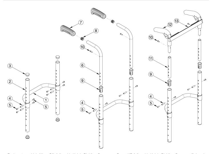
For item 1, see Little Wave Clik Adjustable Height Rigidizer Bar page or Rogue XP Adjustable Height Rigidizer Bar page. If changing from another style backrest and the Drum Brake is present, a new Drum Brake Cable Kit may be required If chair shipped after 7/3/2025 and Rigidizer Mounted Stroller Handles are present, please refer to quote the appropriate Stroller Handle Page for the Rigidizer.
