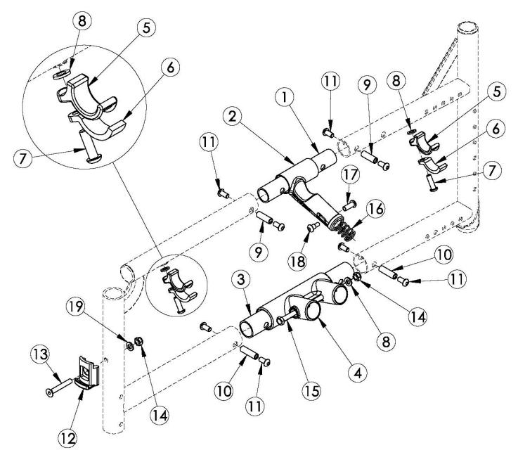
Upper Pivot Assemblies are based on seat width
