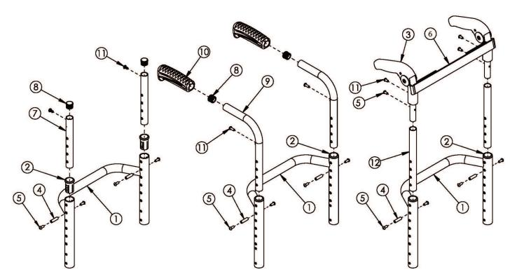
If chair was ordered with Rigid Locking Fold Down Back, please see Rigid Height Adjustable Back Post with Non-Adjustable Height Rigidizer Bar page. This Rogue Style Backrest is not available with the Tsunami Heavy Duty option If retrofitting to this backrest style, a minimum 1" of adjustable depth is required in addition to the Rogue Style Locking Backrest Mount and Hardware.
