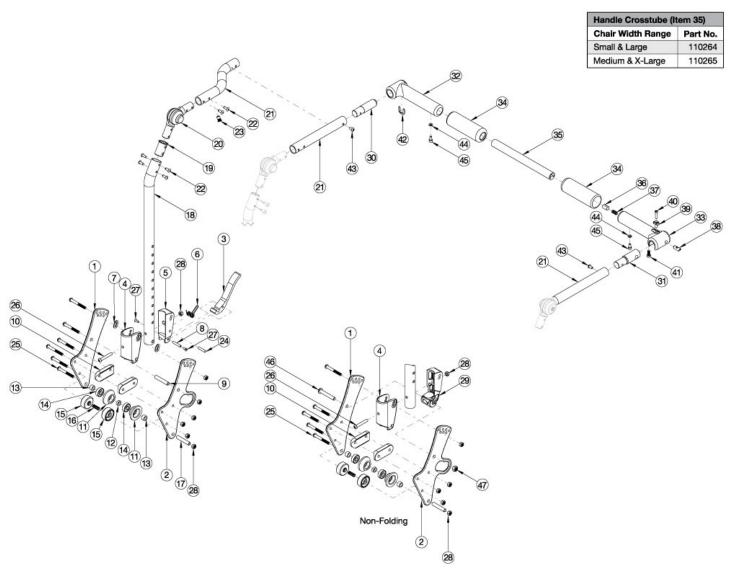
If chair was invoiced prior to 12/18/23, an upper back tube assembly is required. If chair was invoiced after to 12/18/23, parts 18-22 shown in the diagram above can now be purchased individually. Callout #21: The curved tube is used with the small and medium width ranges (10"-14") and the straight shaped tube is used with the large and extra large (14"-18") width ranges. When changing backrest types, check to see if new cables and tilt triggers are needed for both foot and hand tilts.
