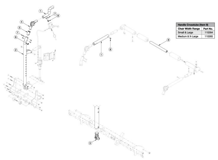
Callout #1: 10"-13" widths receive the curved tube and 14"-18" widths receive the straight shaped tube. When changing backrest types, check to see if new cables and tilt triggers are needed for both foot and hand tilts. If chair was invoiced prior to 12/18/23, an upper back tube assembly is required. If chair was invoiced after to 12/18/23, upper back tube assembly parts can now be purchased individually
