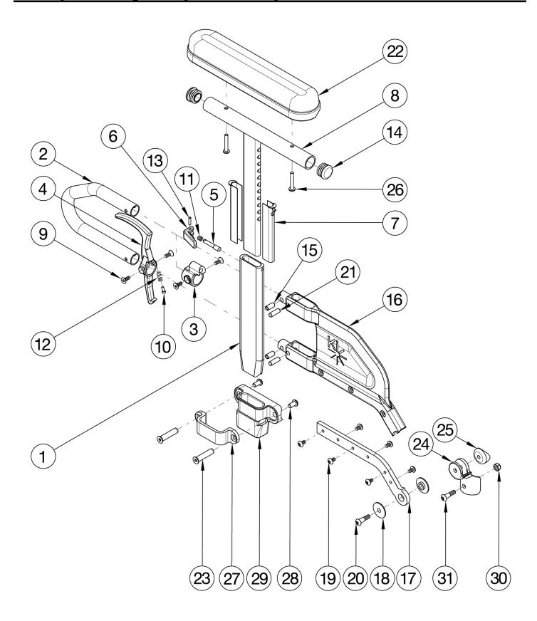
Receiver and Hardware update effective 11/25/24 Short Side Shield used with 14"-17" Seat Depths. Long Side Shield used with 18"-20" Seat Depths. If retrofitting, Receivers are needed.
