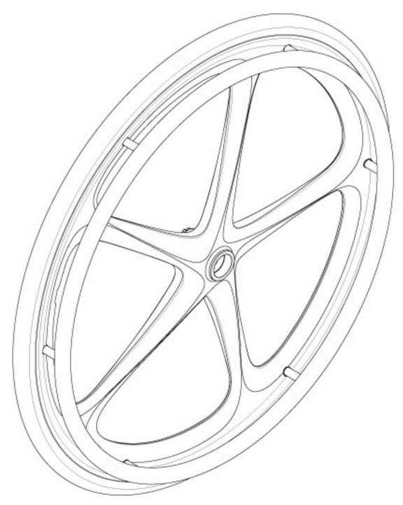
Not all components of the Wheel, Tire and Handrim kits will be listed. These kits cannot be used if Drum Brake is present. If changing wheel size and anti-tips are present, new anti-tips may be required. If changing wheel size or style, new axles and/or receivers may be needed. New wheel locks might be needed when changing wheel size or style.
