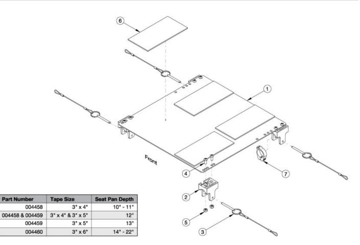
This is an Aluminum Seat Pan for Transit Use. Requires Seating System Cross Braces. The width and depth of the seat pan will measure approximately 0.5" shorter than the listed description.
