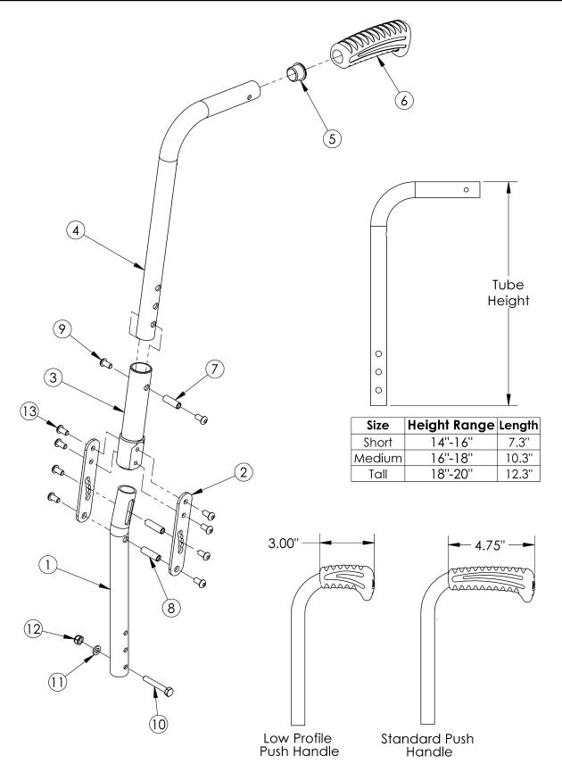
Low Profile Push Handles are not available with Heavy Duty Option or Drum Brake If changing from another style backrest and the Drum Brake is present, a new Drum Brake Cable Kit may be If Anti-Rollback is present, see Back Tubes for Anti-Rollback System
