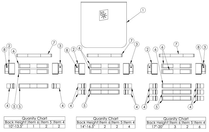
Open Back Panels are used when integrated push handles are present. Closed Back Panels are when backposts without push handles are present. Tension Straps (7a-7b) are used with the combination of Fold Down Push Handle and Tension Adjustable Back Upholstery. Tension Straps 6a, 6b, 7a and 7b are based on chair width.
