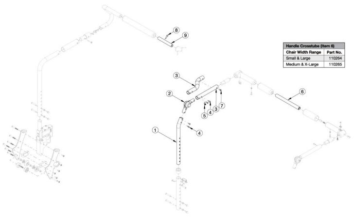
Callout #3: 10"-13" widths receive the curved tube and 14"-18" widths receive the straight shaped tube. When changing backrest types, check to see if new cables and tilt triggers are needed for both foot and hand tilts. If chair was invoiced prior to 12/18/23 and if a Height Adjustable Backrest is present, an upper back tube assembly is required. If chair was invoiced after to 12/18/23 and if a Height Adjustable Backrest is present, upper back tube assembly can now be purchased individually
