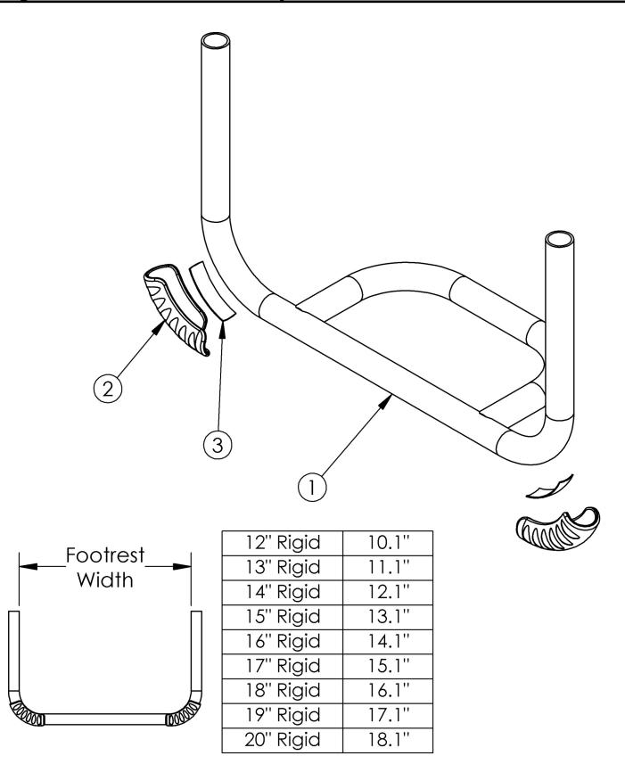
Not available with V-Taper options. Sizes based on straight frame. If changing from a high mount footrest to a frame inserted footrest, please see the "Rogue2 Rigid Frame" page for necessary attaching hardware.
