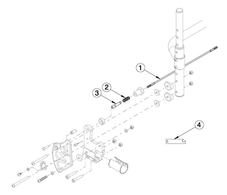
Back Release Cable based on seat width The Back Release Cable length will measure 1" less than the specified seat width
