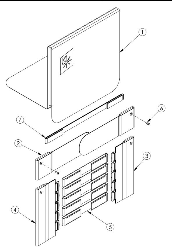
Tension Straps (7a-7d) are used with the combination of Fold Down Push Handle and Tension Adjustable Back Upholstery.Tension straps (5a-5d and 7a-7d) are based on chair width.
