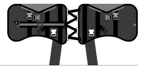
• Turn the harness over (the coloured inside should be facing upwards) and ensure the groin straps are lying out straight. The harness is now ready to use.
