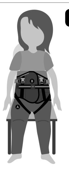
Warning – if the harness slips during use it may not be properly secured. Start the process of donning the harness again rather than trying to correct this when the user is upright.
