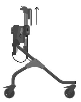
Once the shoulder unit is in the desired position, flip the grey lever down again to lock.
