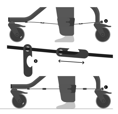
• To detach the ankle guides, release the ankle guide pad from around the user and loosen the knob at the end of the frame tube to pull the screw out through the hole. Unloop the ankle guide from the crevice between the front castor and frame tube. Repeat with the other pad and ankle guide.
