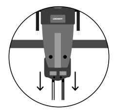
If the frame is at a low height and the pulley straps are hanging down, you can attach them to the clips at the bottom of the framethis ensures the straps are out of the way.
