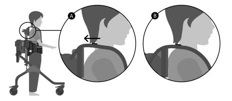
• If, after the harness has been attached to the frame, the user appears to be slipping through the straps, the shoulder straps can be positioned across the user's body. Cross the shoulder straps across the front of the user's body in an 'X' shape then clip each strap into the buckle on the harness which would be on the opposite side from when the shoulder straps and harness are connected in the standard set up.
