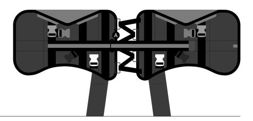
• The stripe belt strap can be folded back and fastened onto the Velcro- this holds the belt in place and ensures there are no obstructions when donning the harness.
