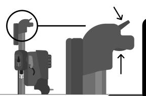
Note – in order to operate the overall height adjustment, the fine height handles need to be in their vertical, foldedaway position. Overall height cannot be adjusted if these handles are facing outwards (horizontal).
