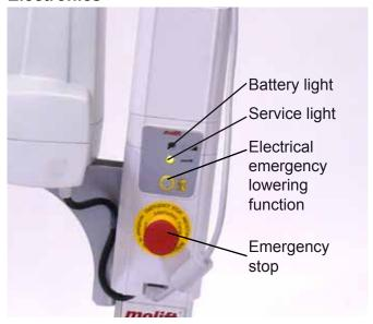
The lift counts the number of lifting manoeuvres performed. This information can be read using the Molift Service Tool, which will indicate when the lift needs a service, e.g. a new lift motor. Please also refer to the Maintenance chapter.
