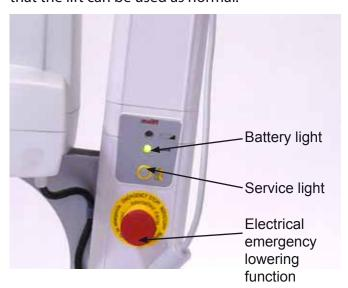
The electronics record the loads lifted and how much the lift has been used. After a certain period of operation a signal is given to indicate that service is required. The service light has the following signals:
