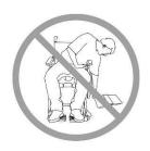
**USERS MUST NOT** position the Jaz-SP on a side slope as this could cause the chair to tip.
