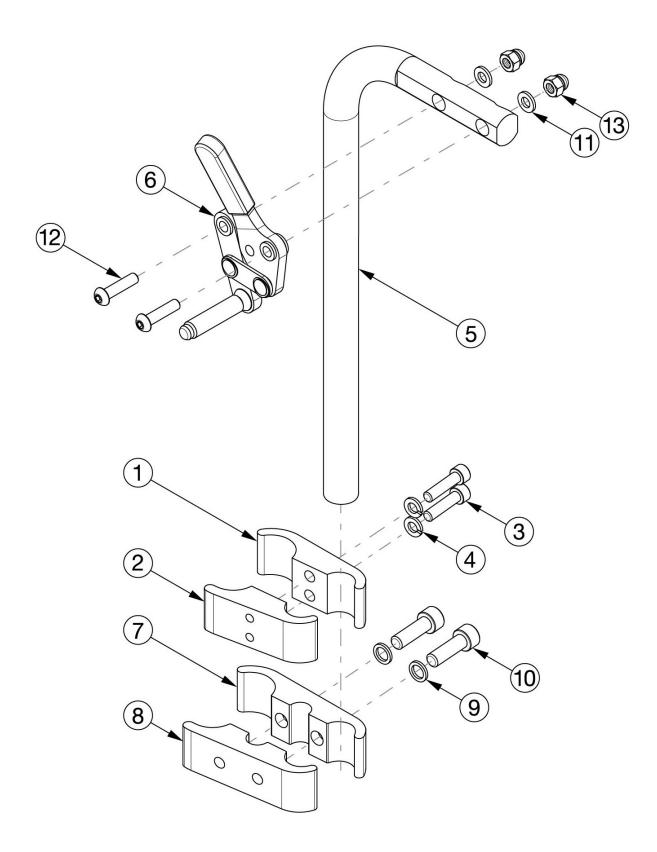
Standard Clamps utilized with 20" wheels in combination with any Center of Gravity positions and 22" wheels in combination with Center of Gravity position 1.
