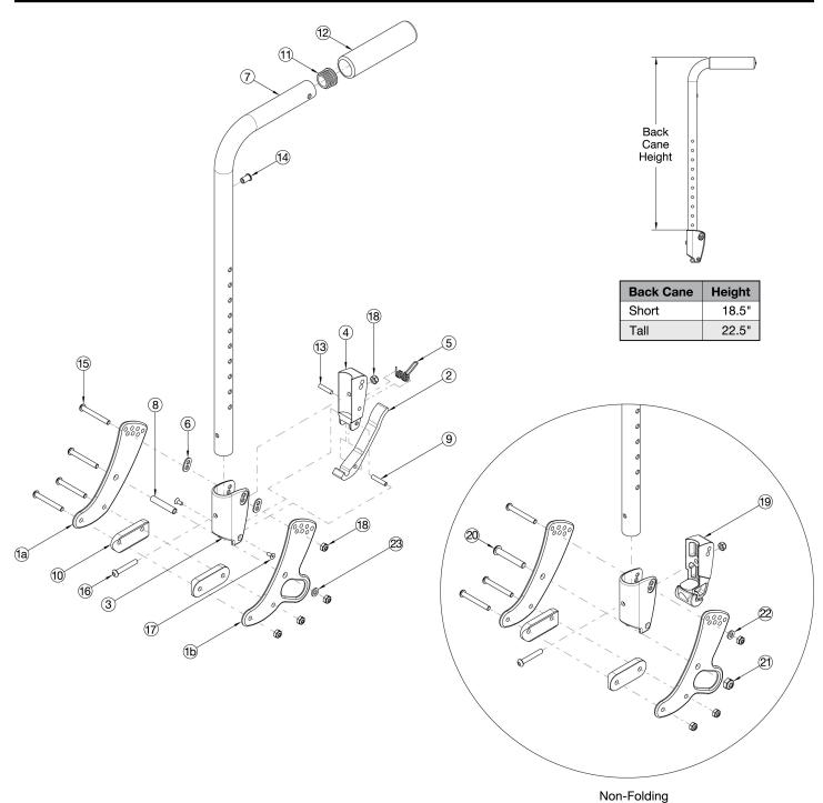
If changing from another style backrest and the hand tilt is present, a new Hand Tilt Cable/Trigger Kit may be required. This design effective starting with serial numbers FCR0026599 and FCHD002333. If serial number is prior to FCR0026599 and FCHD002333 and the hand tilt is present, a new hand tilt mechanism is required in addition to the back cane assemblies.
