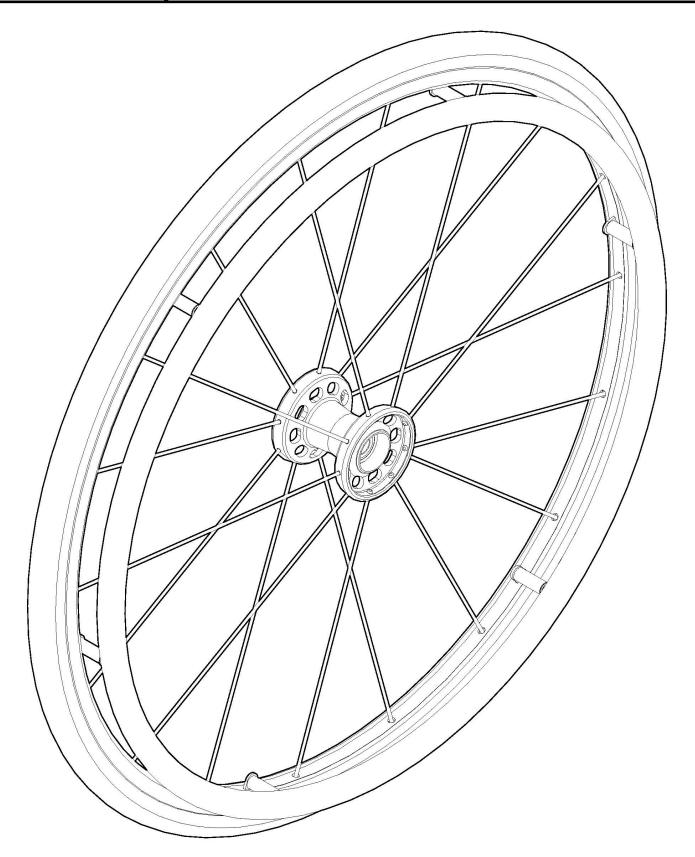
Not all components of the Wheel, Tire and Handrim kits will be listed. These kits cannot be used if Drum Brake is present. If changing wheel size and anti-tips are present, new anti-tips may be required. If changing wheel size or style, new axles may be needed. For Focus chairs, new wheel locks might be needed when changing wheel size or style.
