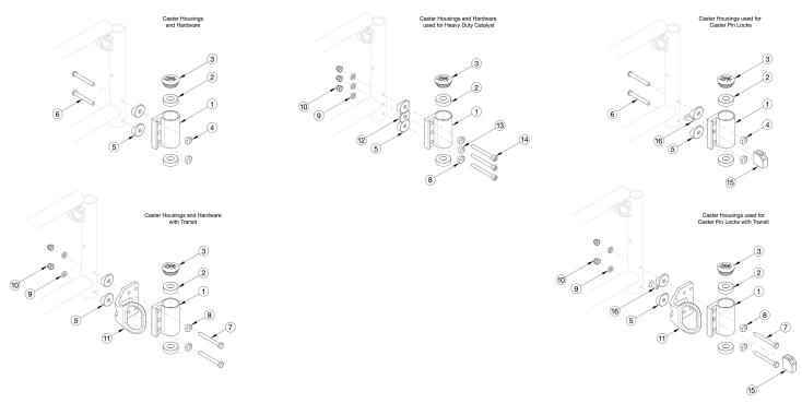
If replacing a caster housing and the chair has caster pin locks, please see Catalyst Caster Pin Locks page. Please Note: The shown orientation of the caster housing above is in the "Forward" position.
