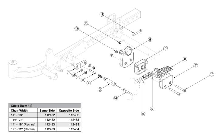
Cables are determined based on width of chair. Please see chart within diagram to determine which cables are used. If retrofitting from Hand Tilt, the complete Foot Tilt Kit is recommended. Cables are determined based on the width of the chair and which side the tilt mechanism is mounted to. If right side mounted, same side = right; opposite side = left.
