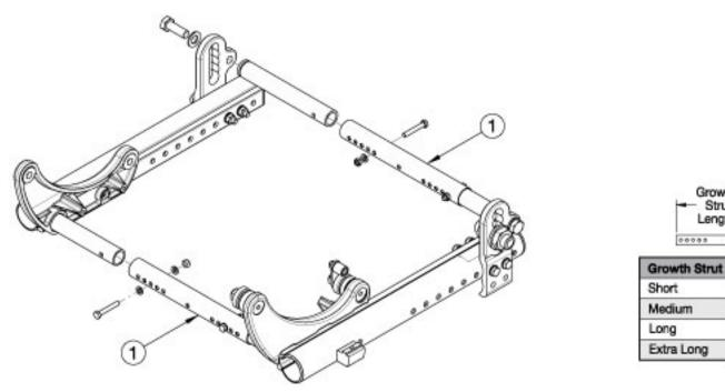
Has your width changed? Will your current base struts work? If not, please select appropriately. To grow the chair, a quantity of two base struts will be needed. One additional base strut is needed if the chair configuration includes an attendant wheel lock. If quoting a Left Frame for Australia or New Zealand, 122921 is required when transit is not present.
