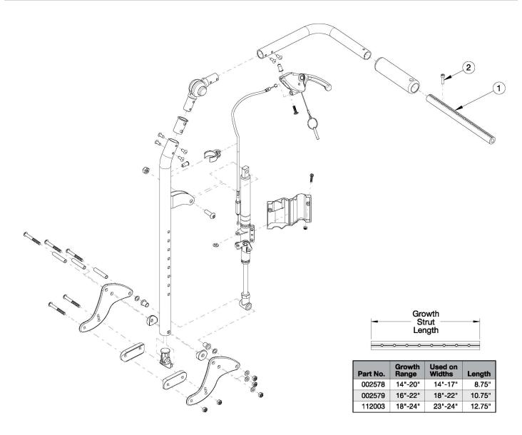
Has your width changed? If yes, verify the current growth strut will work or select appropriately below. If chair was invoiced prior to 12/18/23, an upper back tube assembly is required. If chair was invoiced after to 12/18/23, upper back tube assembly parts can now be purchased individually
