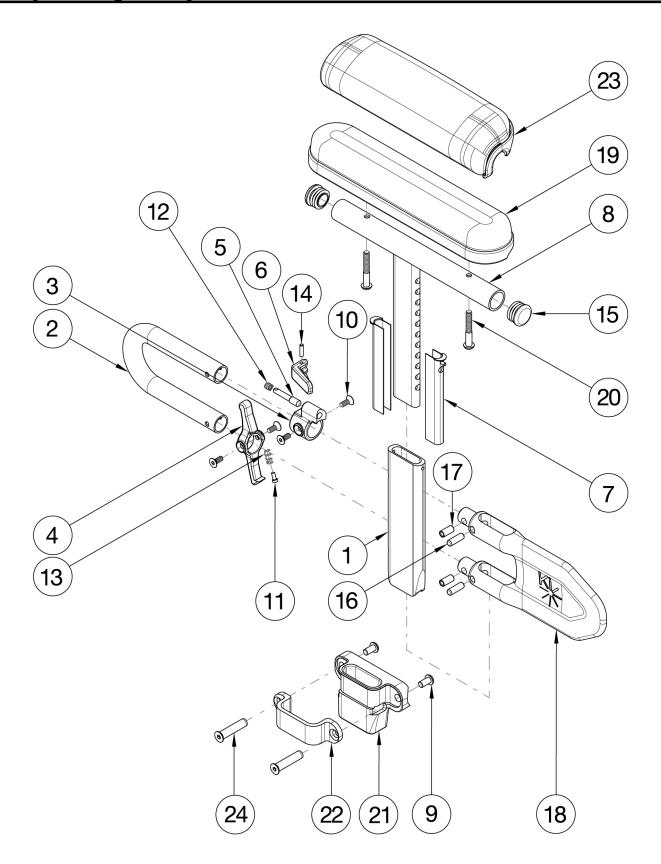
Receiver and Hardware update effective 11/25/24 If retrofitting, Receivers are needed. If retrofitting to Height Adjustable Low T-Arms and One Arm Drive is present, a new drive shaft may be required. In addition to a new drive shaft, order the corresponding hardware kit: 109438 for Blade Style One Arm Drive, 503433 for Hex Style One Arm Drive or 112898 for Quick Release Style One Arm Drive
