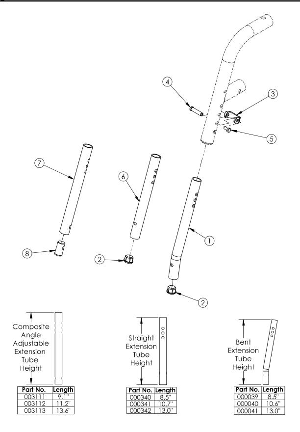
If hangers are being quoted/ordered in addition to extension tubes, fasteners (#3, #4, #5) are already included with the full hanger assemblies (Reference the 60,70,80,90 degree hanger pages). If quoted, composite angle adjustable footplates with hardware extension tube without plug should be quoted.
