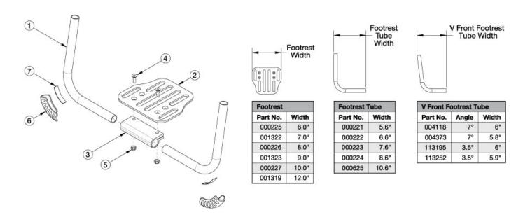
If changing from a high mount footrest to a frame inserted footrest, please see the "Rogue2 Rigid Frame" page for necessary hardware.
