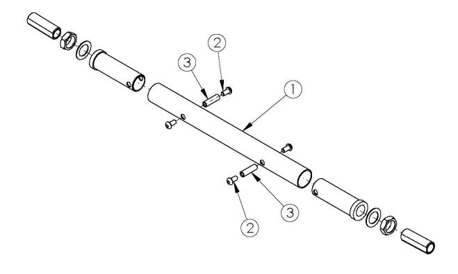
Black Camber Tube kits based on seat width. Color Anodized Camber Tube kits used on all chair widths. New camber tube required when changing the degree of camber by more than 2 degrees. If Wheelchair Drive Ready Option is present, replacement parts need to be processed through Alber USA.
