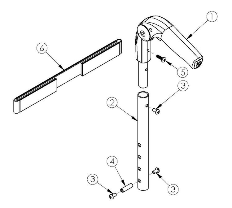
Tension Straps are used with the combination of Fold Down Push Handle Tension Adjustable or Padded Velcro Adjustable Back Upholstery. Straps are based on chair width. Not available with Heavy Duty Option
