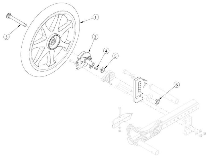
If changing wheel size and anti-tips are present, new anti-tips may be required. If changing wheel size or style, new axles may be needed.
