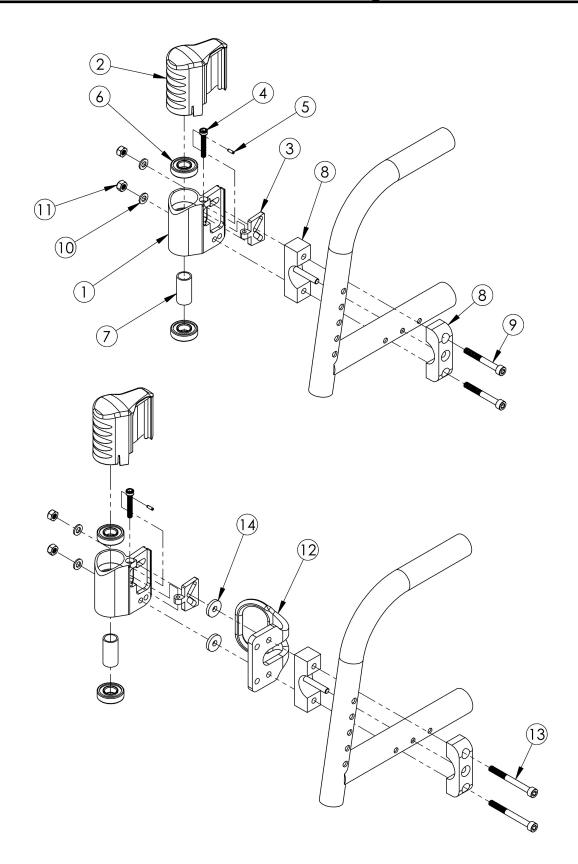
Not Available with Heavy Duty Option Please Note: The shown orientation of the caster housing above is in the "Forward" position. If only 1 side caster housing is needed, customer must confirm the orientation of the caster housing.
