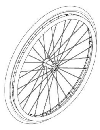
Not all components of the Wheel, Tire and Handrim kits will be listed. These kits cannot be used if Drum Brake is present. If changing wheel size and anti-tips are present, new anti-tips may be required. If changing wheel size or style, new axles may be needed. For Focus chairs, new wheel locks might be needed when changing wheel size or style.
