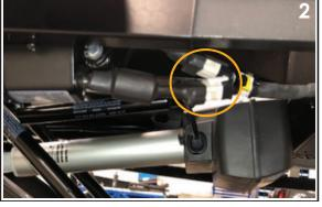
A. Remove PCM Assembly(Continued): 6. There are two locking screws attached to the under side of the two silver pins. (Fig. 7) With a 2.5mm hex key remove both of the locking screws. If it is possible, the locking screws are accessed easier by extending the legrest out or lifting the seat up. Once the locking screws are removed, take a standard screwdriver, and tap both silver pins out and remove the legrest. If the legrest is still under warranty, return to Sunrise Medical. Otherwise discard.
