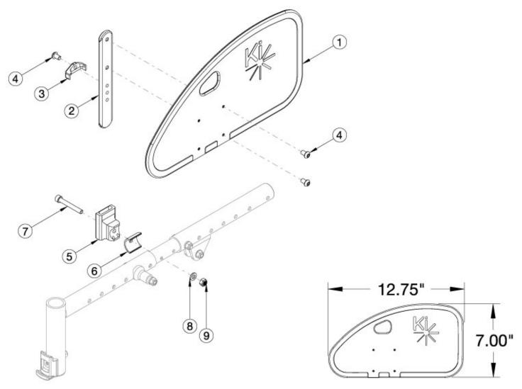
Callout #6: Spacer is needed when the receiver sits on the seat growth tube. Callout #7: Depending upon the placement of the receiver will depend on the length of screw you'll need. More specific information is on the way! Please note there is a receiver screw and spacer kit that includes all potential screw sizes and spacer (you will need qty 2 for a pair).
