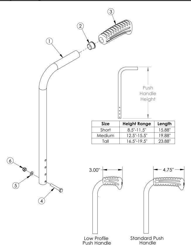
Low Profile Push Handles are not available with Heavy Duty Option or Drum Brake If changing from another style backrest and the Drum Brake is present, a new Drum Brake Cable Kit may be required
