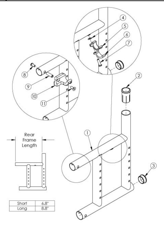
If chair has any type of direct mount side guards, select a frame assembly with Side Guard Mount Modification. Use the short frame for 14-17" Seat Depths. Use long the frame for 18-20" Seat Depths.If switching to a new Seat Depth, new Height Adjustable Flip Back T-Arms may be required.
