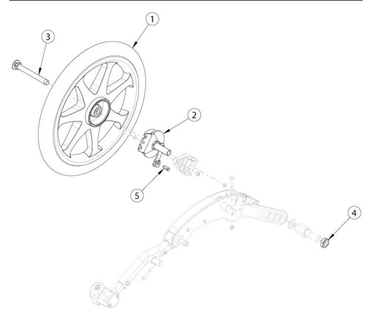
If changing wheel size and anti-tips are present, new anti-tips may be required. If changing wheel size or style, new axles or axle plate and wheel locks may be needed.
