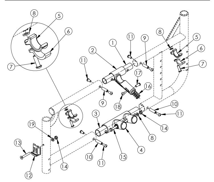
Upper Pivot Assemblies are based on seat width
