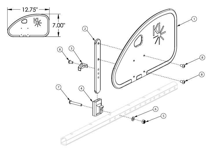
Rear holes on side guard panel (#1) are drilled for all chair configurations, unless otherwise specified. If retrofitting, side guard receivers may be required
