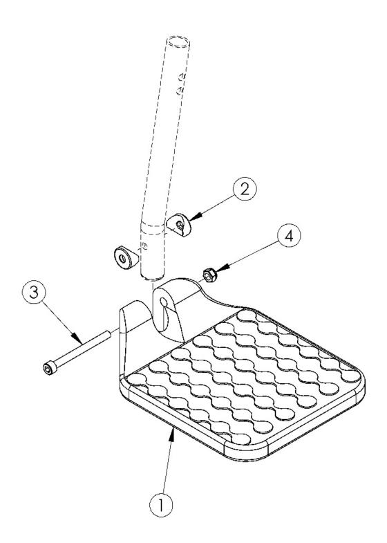
Sizes for footplates are based on seat width with straight frame; if Tilt chair has Offset Frame, add 2" to seat width. If changing footplate style, new extension tubes may be needed. Only compatible with extension tube hangers.
