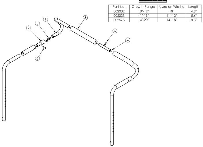
If adding the Removable Stroller Handle to a serial number that did not initially have this option, please order the respective Removable Stroller Handle Assembly and Back Cane Assembly. Removable Stroller Handle assemblies are based on seat width
